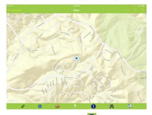
Click the GPS button again to change to a heading mode which will show the location and compass bearing.
